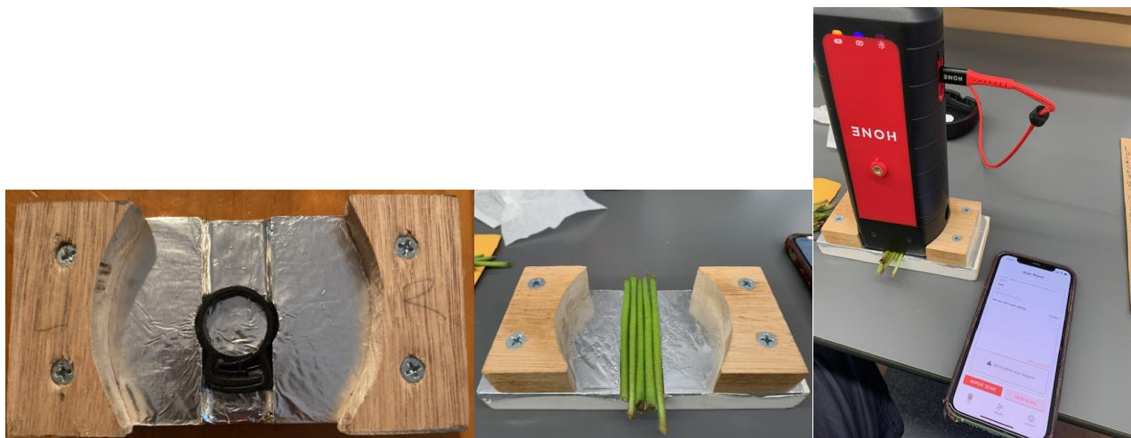
Figure 8. Jig to hold petioles in parallel and in clamped cross-section for accurate capture of spectra. (Developed by Dave McRae)
