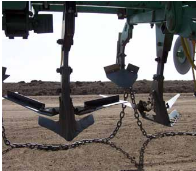
Above Tyne, Sweep and Alabama set up utilized by one grower to develop an “m” profile bed.
